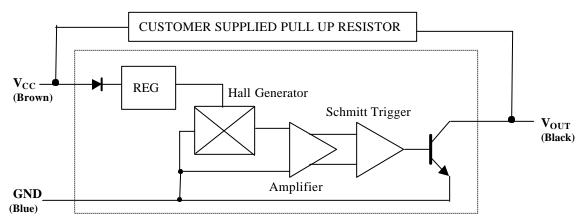
NOTE: A pull-up resistor is required on the open collector output to establish a quiescent voltage level. The pull-up resistor also provides faster rise times and improves noise immunity. Contact the factory for application assistance.
